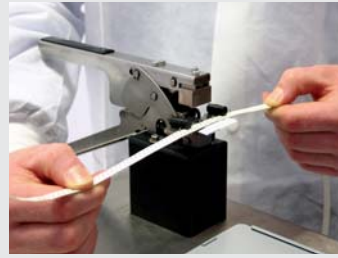
STEP 3 Put depleted reel end into tool, clamp and compress handle of splice tool
